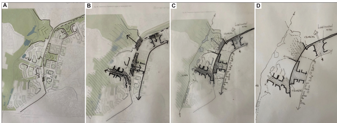
Figure 2. Overlaying on semi-transparent sketch paper during architectural sketching. (A) Visual exploration of patterns; (B) blurring the background and exaggerating remarkable features; (C) formalizing the initial idea into a spatial configuration; (D) abstracted configuration without background. Panels (A–C) show how the original drawing becomes increasingly indistinct.
