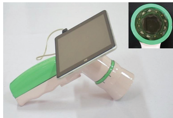
Figure 1. Hand-held CerviScan device developed for cervical cancer detection. The inset shows the front view of the device with the light-emitting diodes positioned around the camera.
