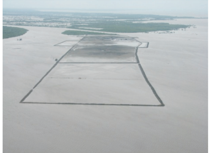
Figure 8: Jetty of 5.2 km length (left) and coastal reclamation area of 40 ha where dredged mud was deposited (right; BPLS, 2011).
