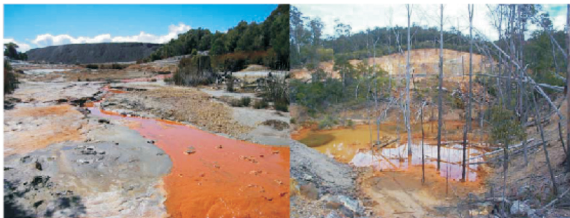
Figure 1. Examples of AMD from the Savage River mine site in Tasmania (left) and from the Strauss open pit at the Mt Carrington mine site in New South Wales (right).
