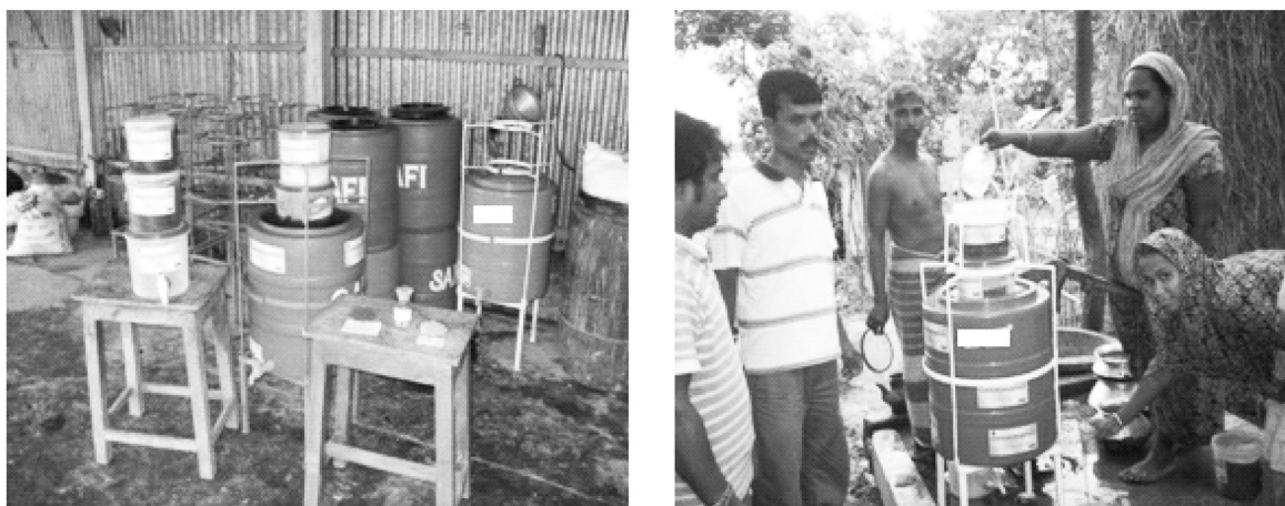
Figure 2: Setup of arsenic filter prepared using NM 4 (left) and a domestic filter (right) in use.
