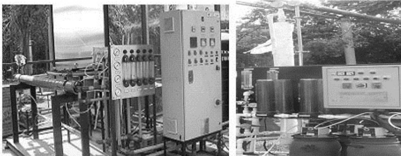
Figure 3: Solar energy driven community level brackish water desalination plant (BARC).
