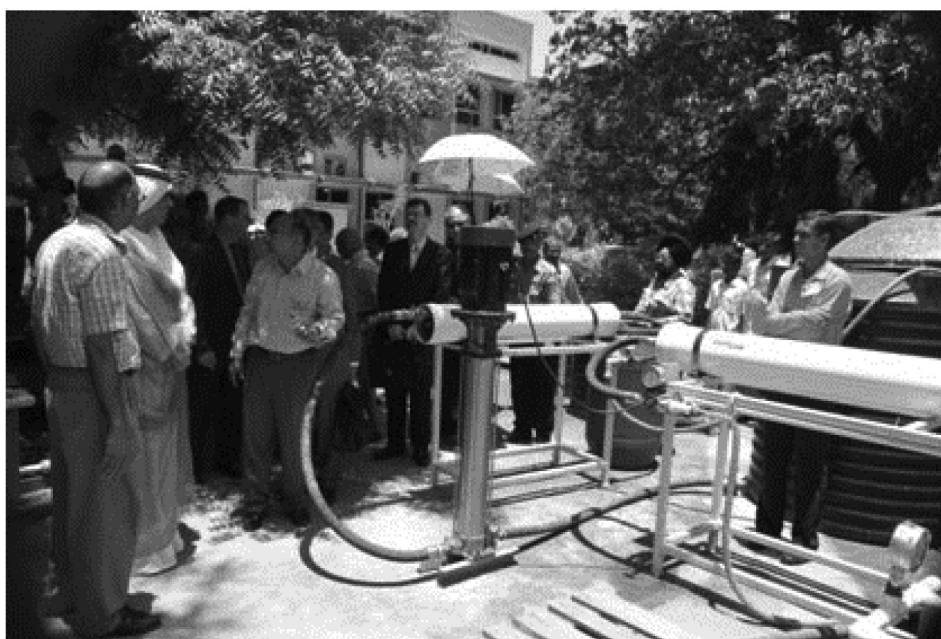
Figure 2: ED-ROM hybrid system high recovery desalination.
