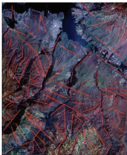
Figure 5: Extracted lineament map from Landsat7 satellite image.
