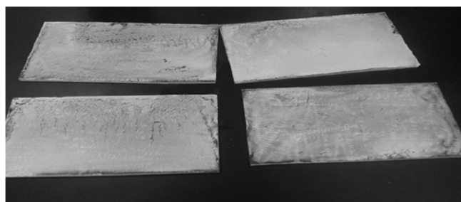
Figure 2: Coated surface of glass with TiO 2 .
