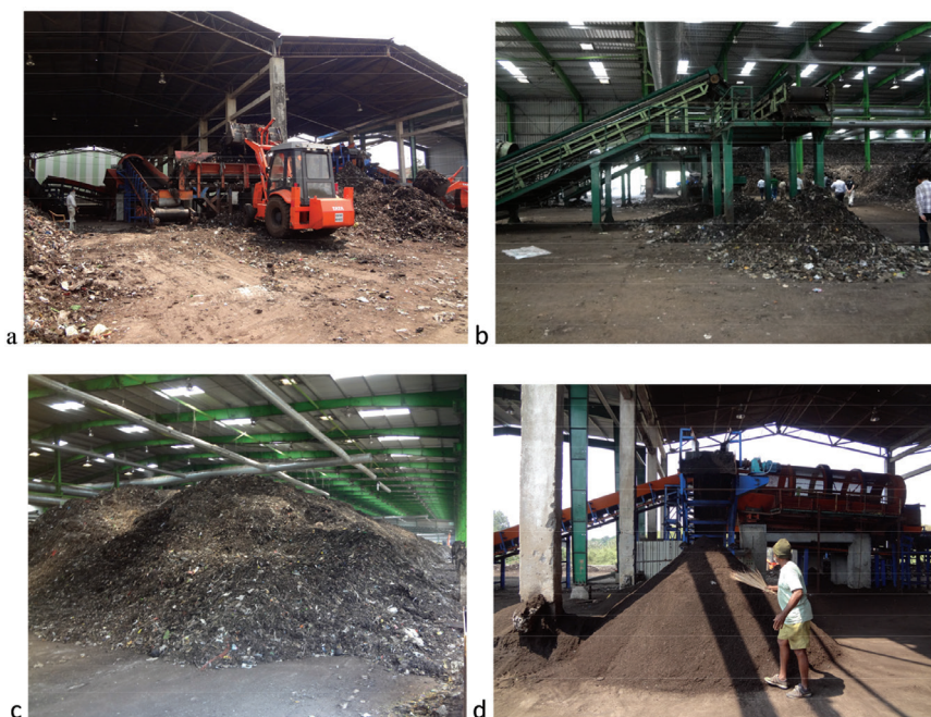
Figure 1: Images of the KCDC plant: (a) MSW receiving area; (b) waste screening through trommel; (c) Windrow composting and (d) Final compost.
