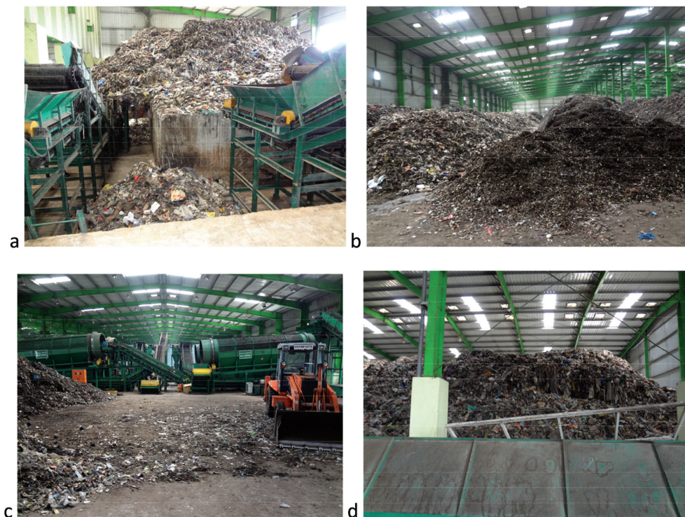
Figure 3: Images of the CMBT plant: (a) Waste tipping floor; (b) Windrow composting; (c) Waste screening through trommel and (d) RdF storage.
