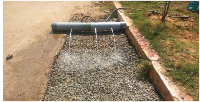
Figure 6: Test set up for lateral discharge.
