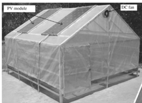
Figure 7: Hybrid PV/T integrated greenhouse dryer (Baranwal and Tiwari, 2008).
