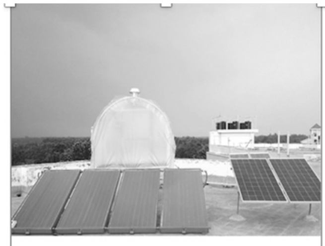
Figure 5: Experimental set up of mixed mode solar dryer (Andharia et al., 2020).
