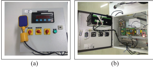
Figure 2: Sensor node hardware setup. (a) Front panel and a level sensor (b) Internal view.
