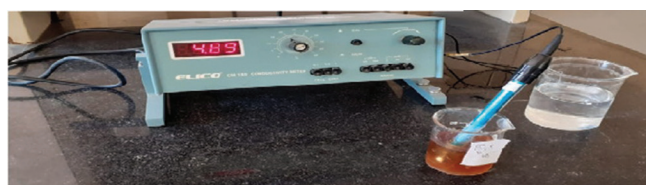
Figure 15: Testing of treated water-conductivity meter.
