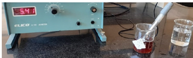
Figure 14: Testing of treated water-pH meter.
