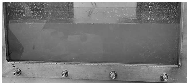
Figure 7: Ultra-fine bubble cloud formed in the pilot scale de-oxygenation tower.
