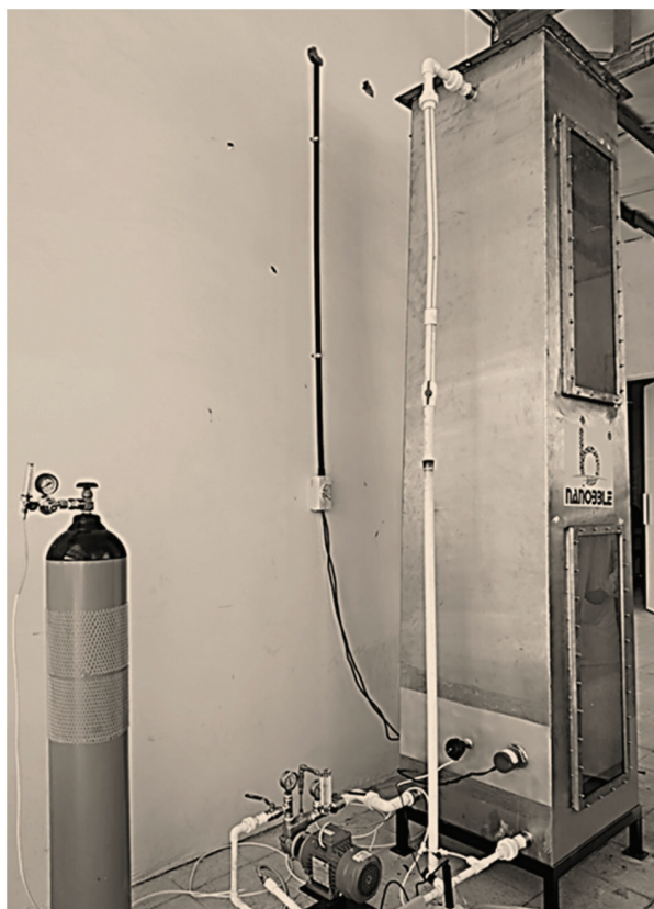
Figure 2: Pilot scale (1.08 m 3 liquid volume) gasification tower equipped with an ultra-fine bubble's pump.
