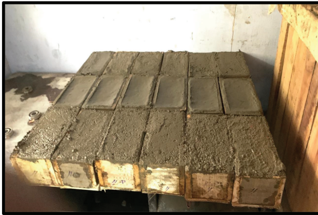
Figure 4: Moulding of brick samples S1, S2, and S3.
