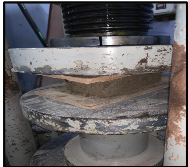
Figure 6: Compressive strength test.
