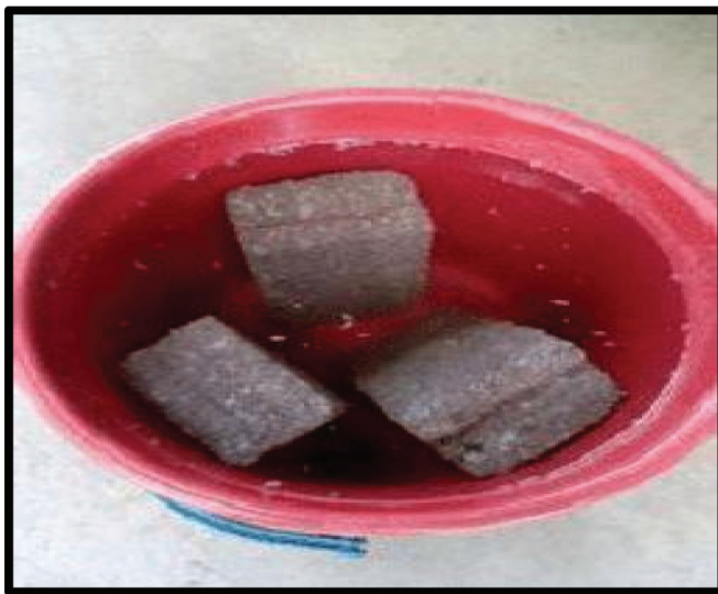
Figure 8: Brick samples are submerged in water to measure water absorption.
