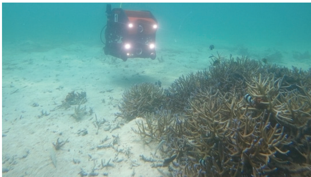
The ROV in use during initial tests to record coral reef imagery in shallow waters. (Photo credit: Raheem D.A., REEF)
