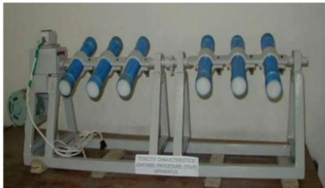
Figure 6: TCLP agitation apparatus.
