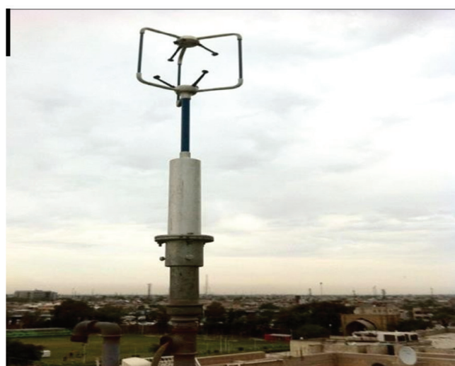
Figure 2: Photograph of 3D ultrasonic anemometer used in this paper.
