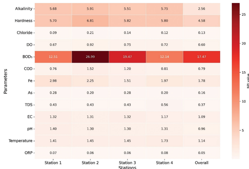
Figure 6. Heatmap representing NPI scores for all samples, with scores above 1 indicating water-polluting factors
