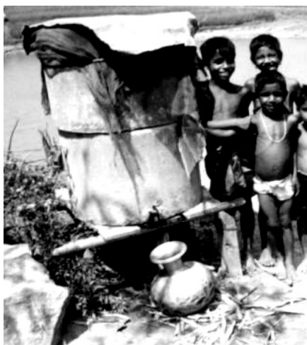
Figure 1: A typical indigenous iron filter unit used in Assam.
