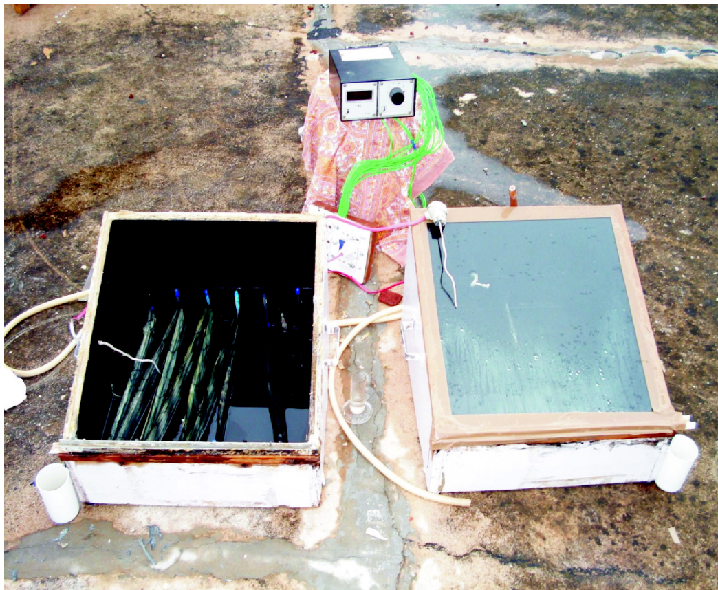
Figure 1: Inside view and top view of still with vertical evaporating surface.
