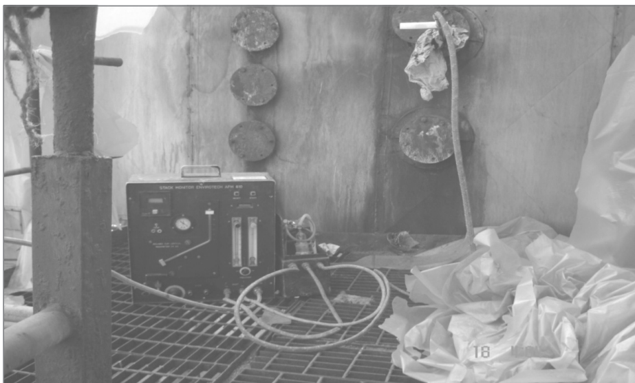
Figure 9: Experimental Set Up by using SO 2 monitoring kit for absorption of SO 2 .
