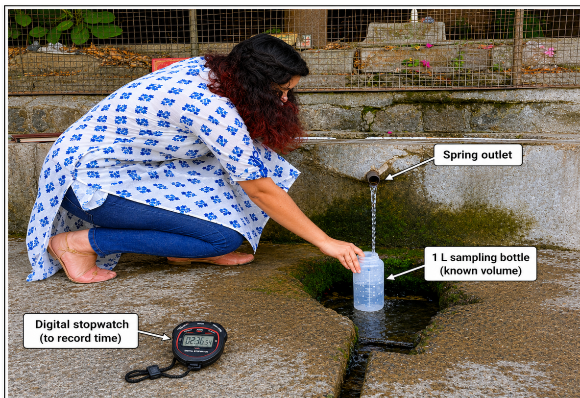
Figure 3. The volumetric method for spring discharge measurement using a calibrated sampling bottle and a digital stopwatch at the spring outlet
