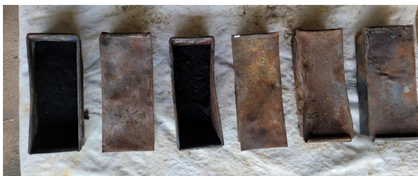
Figure 4. Airtight steel containers used to produce the sawdust char
