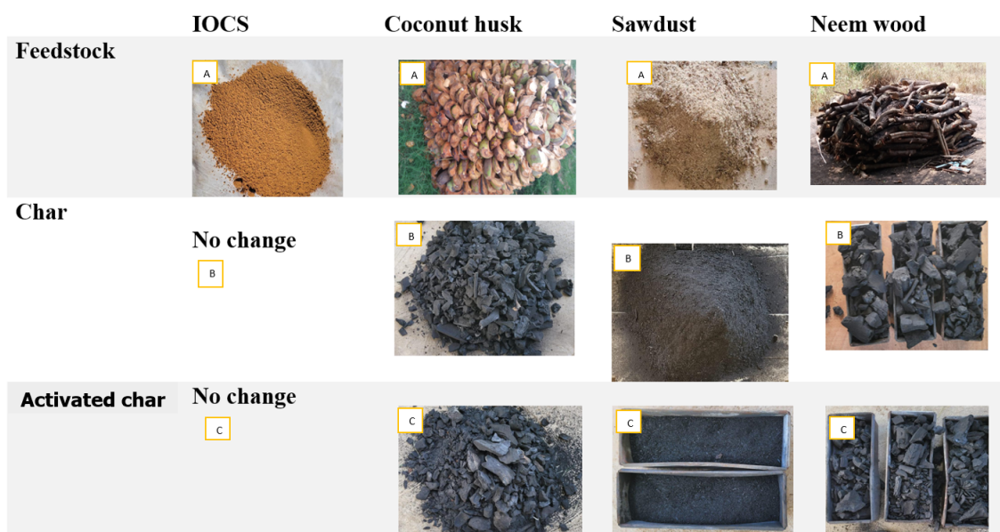
Figure 3. Adsorbent samples used for the study. Various states of the feedstocks: (A) raw, (B) charred, and (C) activated. Abbreviation: IOCS: Iron oxide-coated sand.
