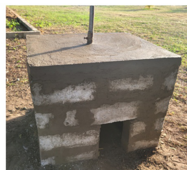
Figure 5. Sketch and picture of the improvised sandcrete/clay oven for char production
