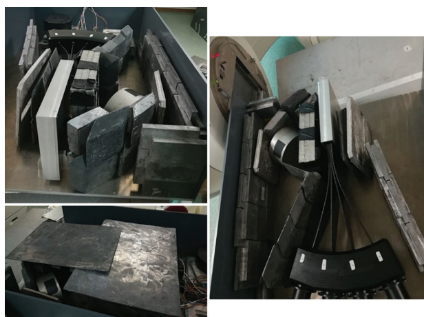
Figure 8. Views from different angles of the shielding configuration employed to mitigate the out-of-field radiation escaping from the linear accelerator (linac) head.
