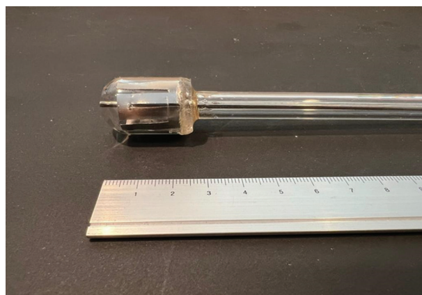
Figure 5. A prototype mini coaxial-type neutron tube. Photo captured by the author.
