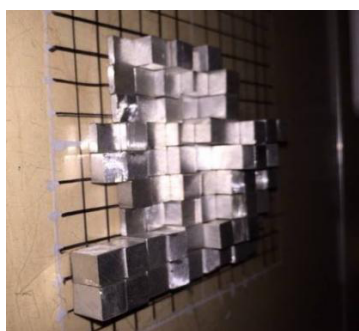
Figure 1. Custom-built aluminum tissue compensator
