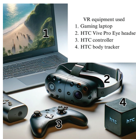
Figure 1. Virtual reality equipment used to assess prospective memory and eye fixation in brain injury survivors.
