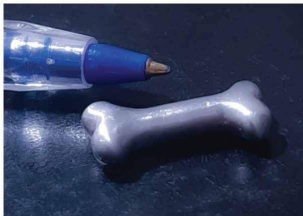
Figure 4. A silver piece manufactured using shell fusion technology
