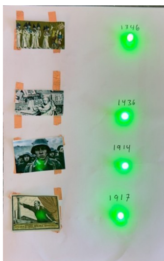
Figure 3. A leaflet with a puzzle design. Each image has a different configuration of copper tape on the back, which completes the circuit and turns on the light-emitting diode only when the event in the image matches the correct date.
