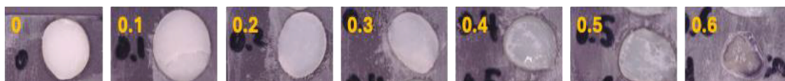
Figure A1. Representative PLA-PUA polymeric blend samples printed at a fixed exposure time of 60 s under seven inhibition ratios: I_{UV}/I_{Blue} = 0 (pure blue), and I_{UV}/I_{Blue} = 0.1, 0.2, 0.3, 0.4, 0.5 and 0.6
