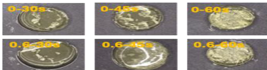
Figure B1. Hydrogel samples printed with and without inhibition for pure blue light ( I_{UV}/I_{Blue} = 0 ) (top row) and a chosen inhibition ratio ( I_{UV}/I_{Blue} = 0.6 ) (bottom row) across three exposure times: 30, 45 and 60 s
