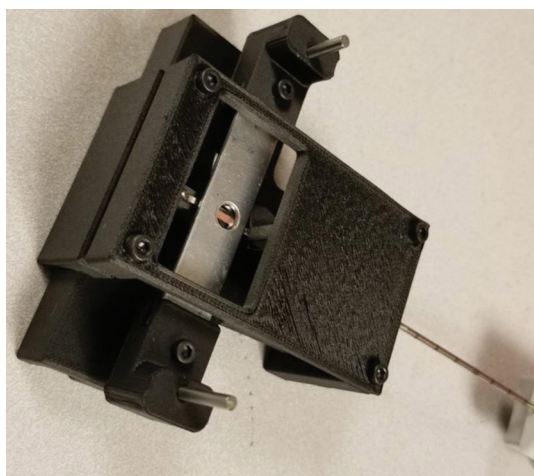
Figure 4. Compression testing device. This simple device enables quantitative assessment of tissue deformation while maintaining histopathological integrity.
