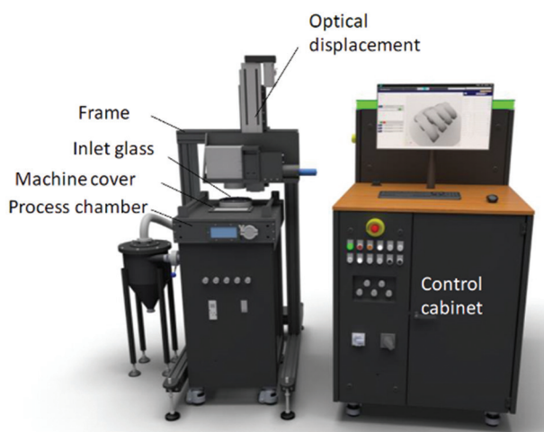
Figure 2. AconityMINI 3D printer utilized for the presented study to produce the sample and record the melt pool temperatures 1 .
