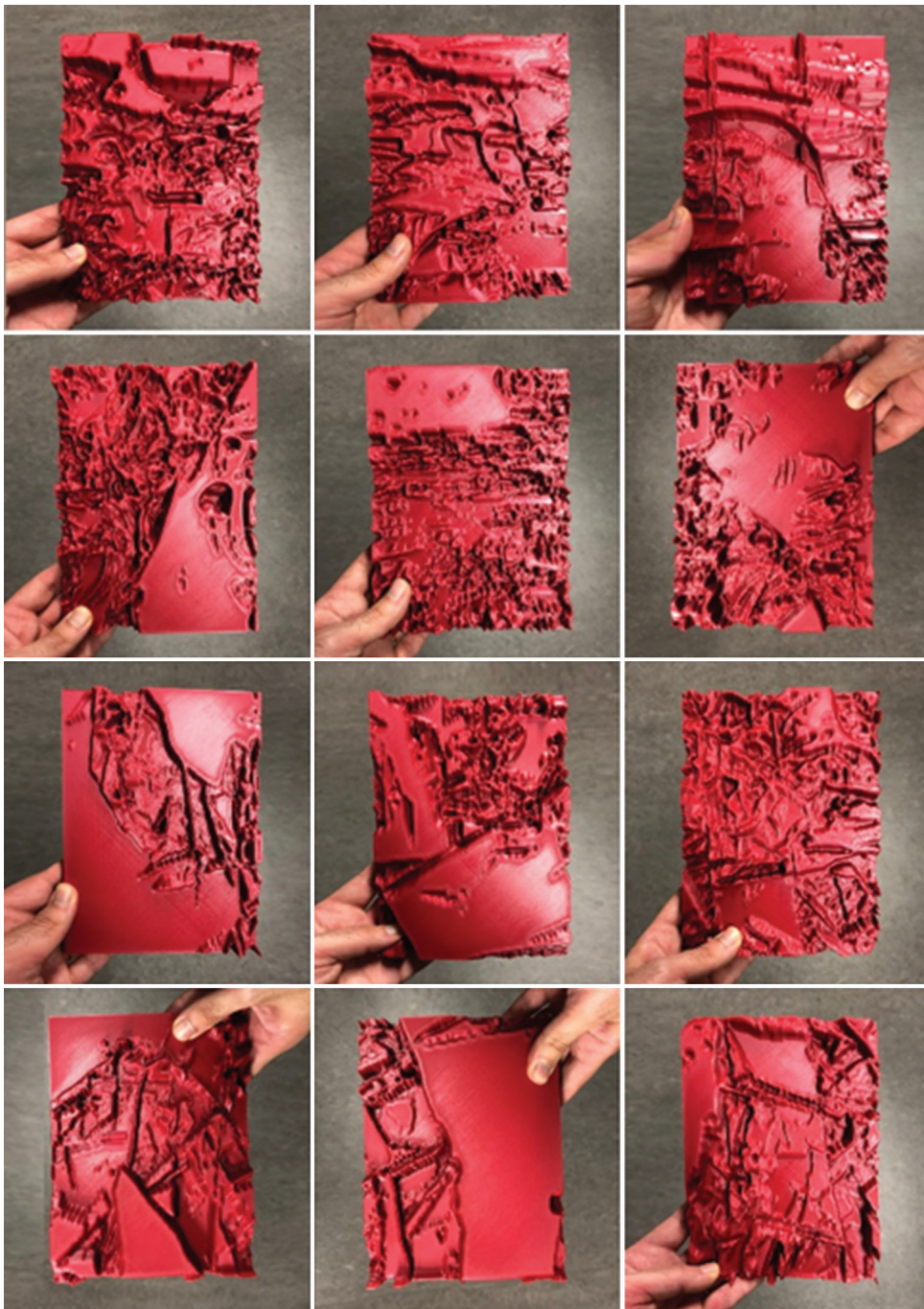
Figure 14. Set of 12 counter-mold parts produced through three-dimensional printing being poured over the assembly (Figure 15). 34
