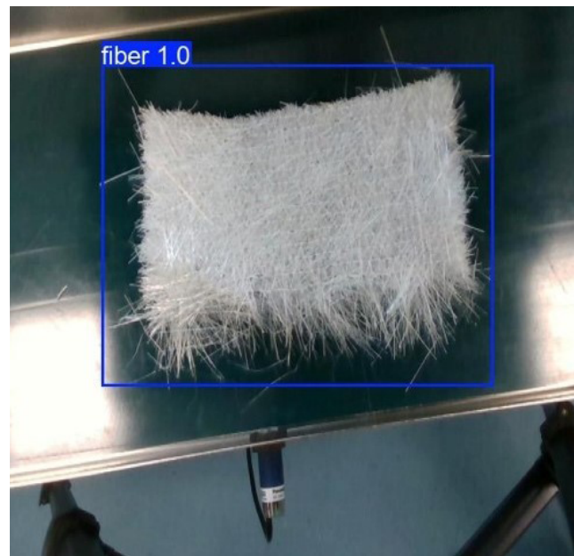
Figure 2. Detection of fiber through RGB image recognition and a convolutional neural network detection algorithm. Image created by the authors.
