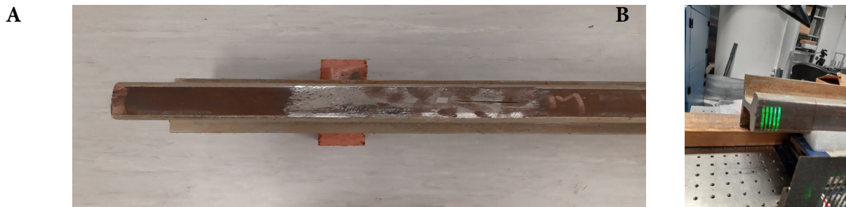
Figure 1. Rail-track specimens: (A) specimen with surface crack; and (B) specimen with incident line arrayed pattern of laser beam for generating narrowband Rayleigh-guided wave.
