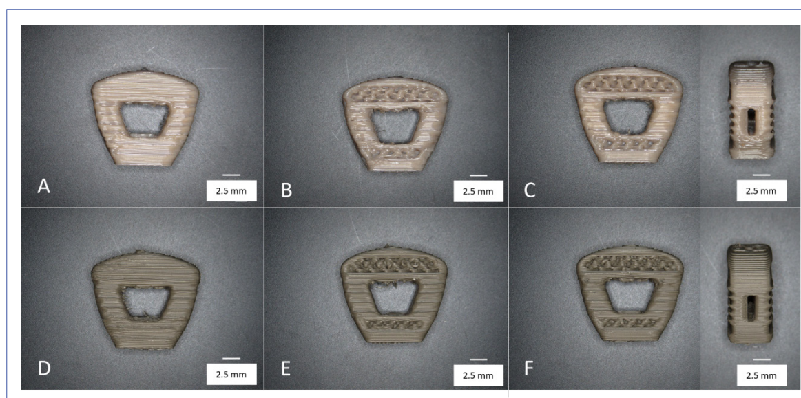
Figure 2. Sample cages that were 3D-printed for mechanical testing. Solid (A, D), porous (B, E), and porous window (front and side views) (C, F) designs for PEEK (A, B, C) and \text{Si}_3\text{N}_4 -PEEK (D, E, F) materials.
