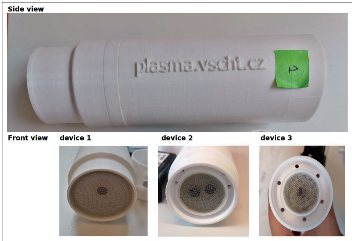
Figure S1. Photographs displaying the external appearance of 3D-printed cold atmospheric plasma (CAP)-generating devices: side view (top) and front view (bottom). Device 1: original version; Device 2: optimized version enclosed in a chamber with a double discharge; Device 3: XXX. The optimized devices (i.e., devices 2 and 3) have holes around the discharges to enhance air and particle flow. They also feature a wall that separates the discharge part from the airflow, making the discharge chamber smaller and the particle atmosphere more concentrated.
