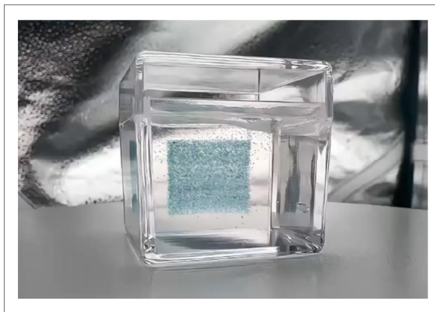
Figure S4. CGC bioink can also be utilized to print patches with intricate-curved surfaces within a suspended medium. Abbreviation: CGC: Conductive granular composite.
