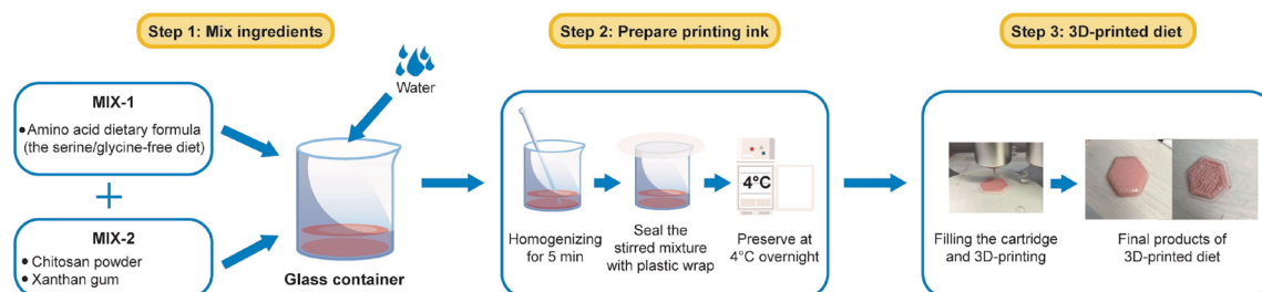
Figure 1. The processing steps from raw materials to the final 3D-printed serine/glycine-free (–SG) diet. Schematic diagrams show the preparation process, including mixing, hydration, and printing. The photographs of the final 3D-printed –SG diet sample show its solid hexagonal prism geometry designed for swallowing assessment.
