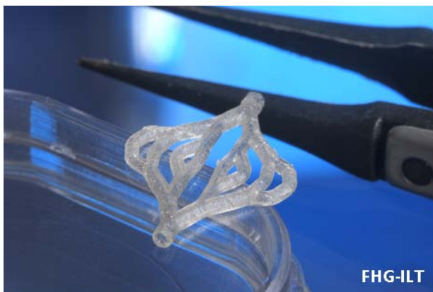
Figure 3. Vessel structure created using stereolithography.
