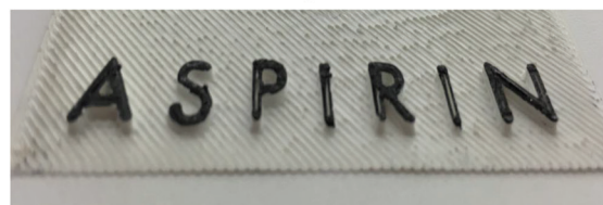
Figure 2. Process of creating the 3D-printed medication label.
