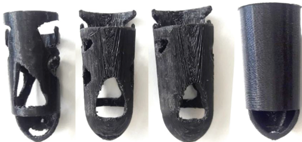
Figure 8. From left to right 62.51%, 71.13%, 79.49%, and 100% mass splints.
