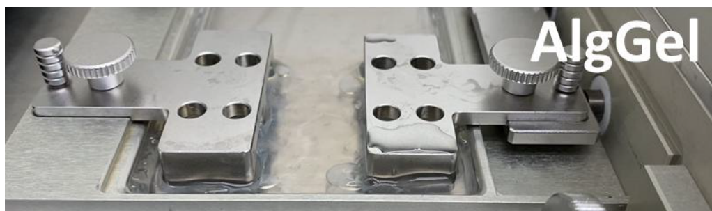
Video S2. Fatigue testing of printed AlgGel patches. The image is a representative illustration of the AlgGel patch behavior, under cyclic loading using Taihoya instrument. The test was performed for 24 h by setting the instrument to 20% dynamic stretch and 60 bpm (which mimics conditions of a healthy human heart). Abbreviations: Alg: Alginate; Gel: Gelatin.
