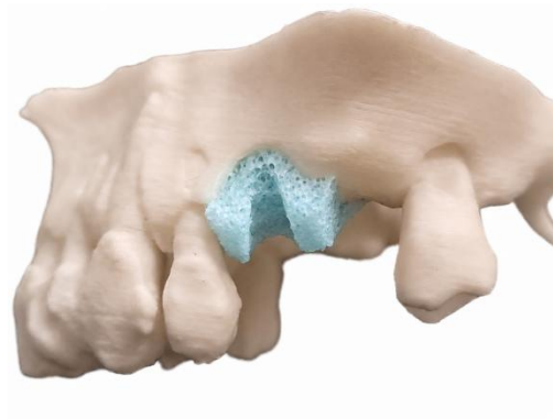
Figure 8. Scaffold fabricated by SLA with Dental Model Water-Washable resin positioned on a patient-specific PLA bone replica.
