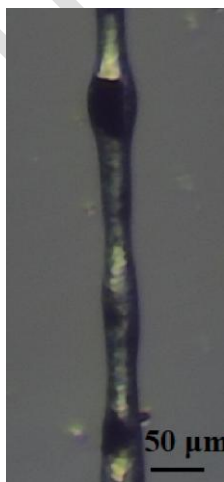
Figure S2. Bead-on-string morphology of 7 wt% PCL/MXene fibers at 50 \mu m target diameter.
