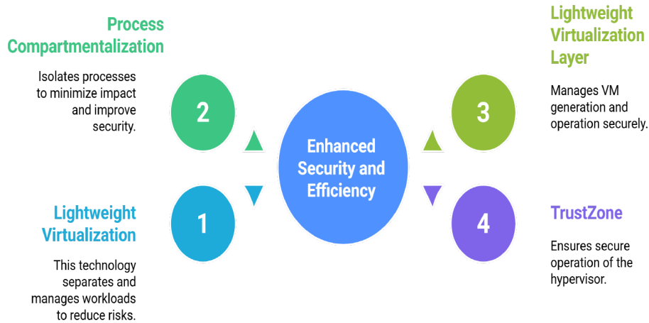
Figure 4. Enhancements of IoT edge device security and efficiency with a lightweight virtualization approach
