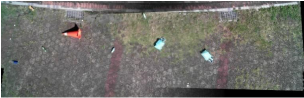
Figure 28. Image stitching using ORB+FLANN+PROSAC with weighted fusion.
