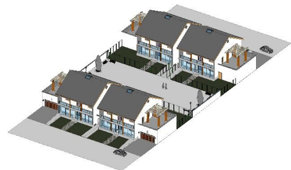
Figure 20. Proposed new courtyard-garden housing compound hosting four nuclear families. Each unit is 240 sqm with 2½ levels above the ground and a semi-basement. Source: Zhang (2015/2017, 2016, 2017) [4,33,34]
