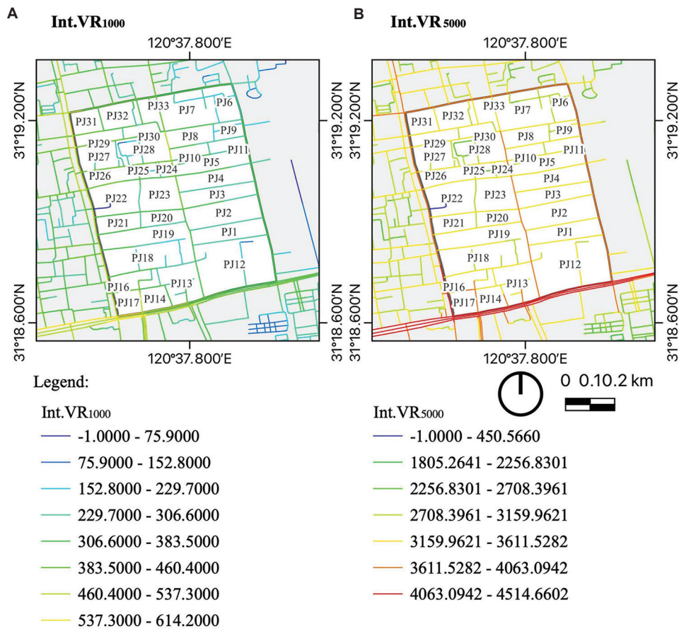
Figure 3. Pingjiang historic district spatial topology analysis diagram. (A) Life integration (Int.V R1000 ) analysis map of Pingjiang historic district. (B) Global integration (Int.V R5000 ) analysis map of Pingjiang historic district. Source: Drawings by the authors
