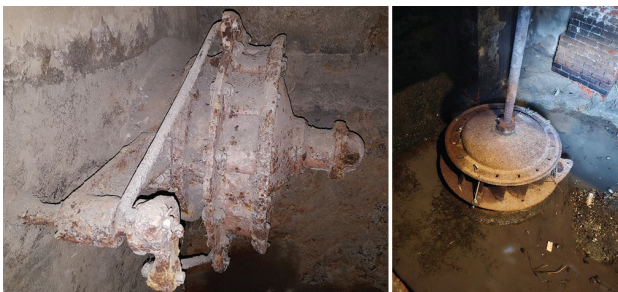
Figure 2. Examples of the open-flume horizontal and vertical-axis Francis turbines. Left: The excavated open-flume horizontal-axis Francis turbine from the water shaft of the Shanping hydropower plant (Deng, 2021). Right: The open-flume vertical-axis Francis turbine in the old Donghai Rice Mill (Wang, 2010).
